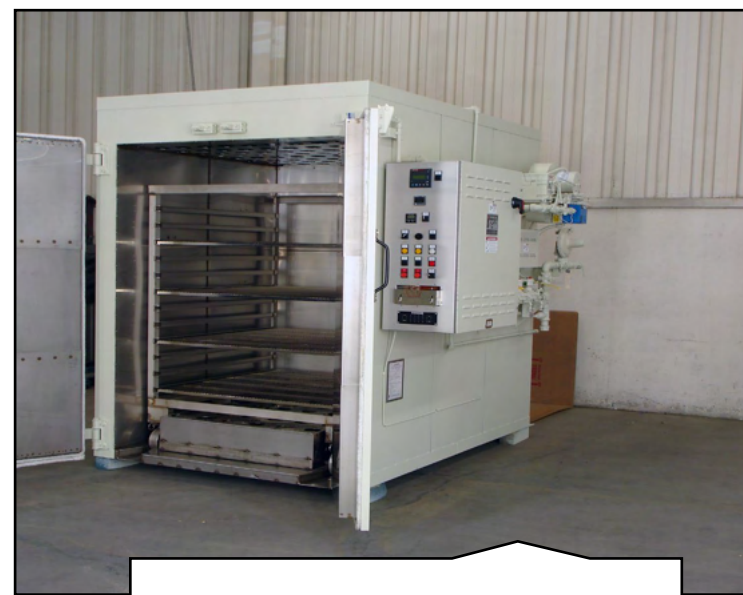
1003 Custom Walk In Ovens Vertical Airflow
