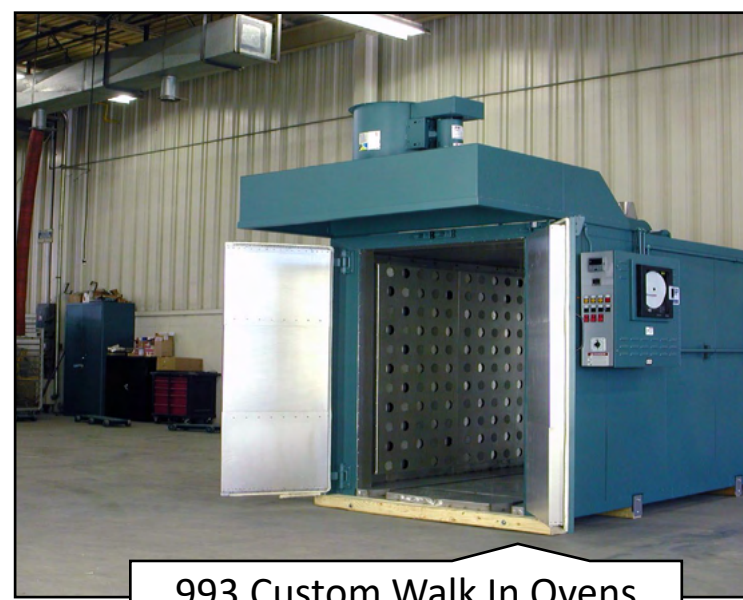
993 Custom Walk In Ovens Exhaust Hood Horizontal Airflow
