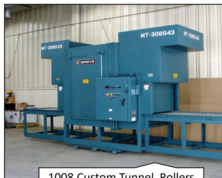
1008 Custom Tunnel Rollers and Roller Rails Vertical Lift Door
