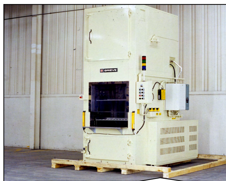
904 Custom Vertical Conveyor Humidity
